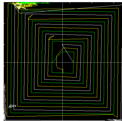
Fig. 1. Representation of three rovers implementing one interlocking spiral, each different color spiral in the graph represent an individual rover.
